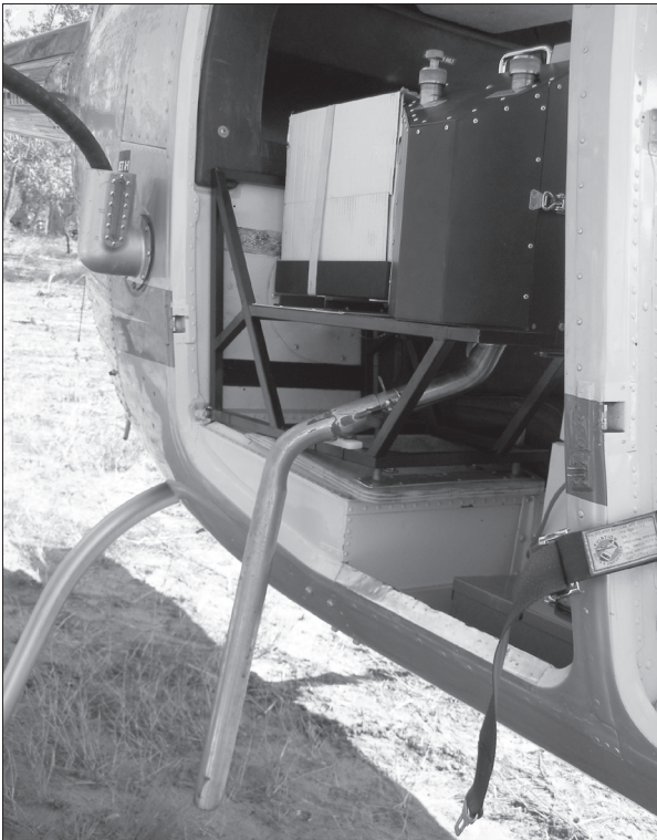
Plate 4: Aerial incendiary device attached to Jawoyn chopper. Source: Lendrum (2007).
