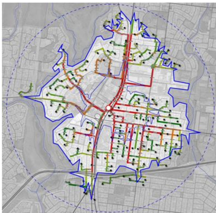
Figure 15 Potential trip numbers calculated in a GIS package (Source: Transport Victoria 2011, p.42)
